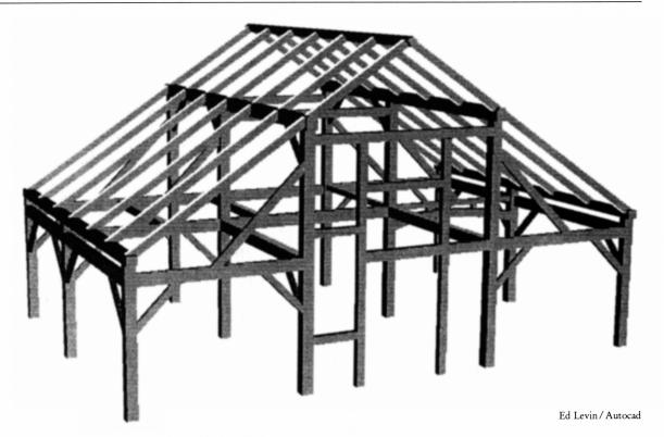
Machine perspective drawing of proposed frame designed by the Guild for the Habitat house. An alternate version will use common purlins instead of the common rafters shown here. More drawings appear on page 3.
